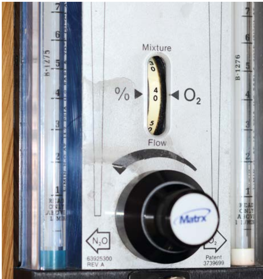
Figure 2 (Left) MDM with cleaning damage
